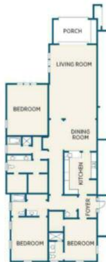
before The kitchen and dining room were located in the interior, ignoring the view.
